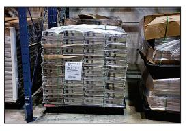
Sheets of cardboard or suitable binder sheets placed between layers will keep the inserts flat.
