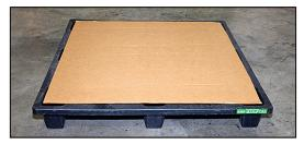
A protective cover should be placed on the pallet before stacking to minimize the possibility of damp or curled sections.
