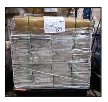
An example of a correctly shipped pallet.
