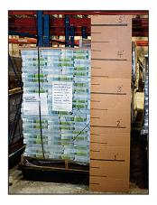
Maximum allowable loaded pallet height is 5 feet measure from the floor to the pallet top.
