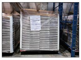
Brick stacking stabilizes the load for ease of shipping, handling and storage.
